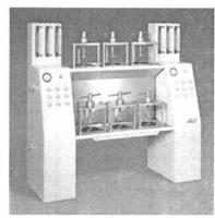
accepts 6 specimens, with quantitative water permeability testing CodeCN820 Weight (kg)120 Tariff902480 9 For testing of concrete test specimens with the following dimensions:
