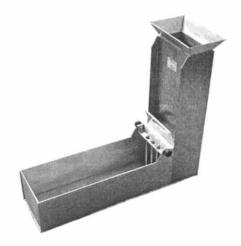
Used for determining the passing ratio of self compacting concrete.
