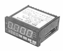
The instrument provides isolated auxiliary power(regularly 5V/80mA) which allows 1-4 loadcells connection directly. Up to 6 outputs control are available for group ingredients weighing or fast/slow weighing; Data/Peak value holding function for choice.
