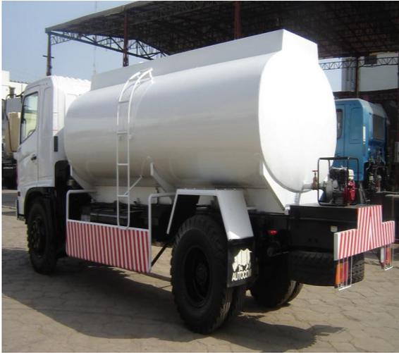
**General:** 10,000 liter water bowzer with pumps (PTO). The tank is constructed of galvanized steel for corrosion protection.
