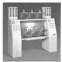
accepts 6 specimens, with quantitative water permeability testing CodeCN820 Weight (kg)120 Tariff902480 9
