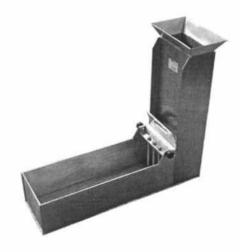
Used for determining the passing ratio of self compacting concrete.
