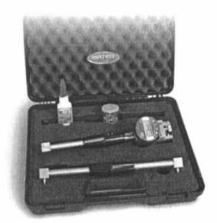
Used to determine the strain (length changes) in concrete specimens and structures, rock strata, different parts of a structure, in remote areas and under adverse conditions, using a single instrument.
