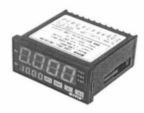
The instrument provides isolated auxiliary power(regularly 5V/80mA) which allows 1-4 loadcells connection directly. Up to 6 outputs control are available for group ingredients weighing or fast/slow weighing; Data/Peak value holding function for choice.
