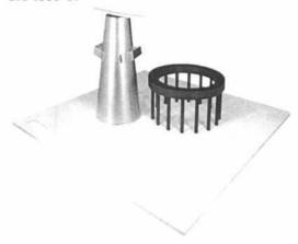
The J-Ring Test Set is used to characterize the ability of self-consolidating concrete (SCC) to pass through reinforcing steel. The test is useful for both mixture qualification and quality control testing.
