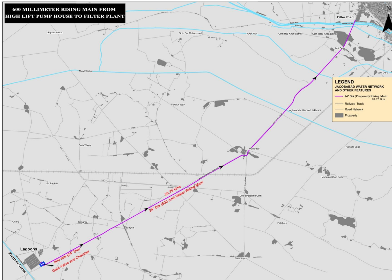
Figure 3: Route Plan 600 mm Rising Main from High Lift Pumping Station to Water Filtration Plant.
