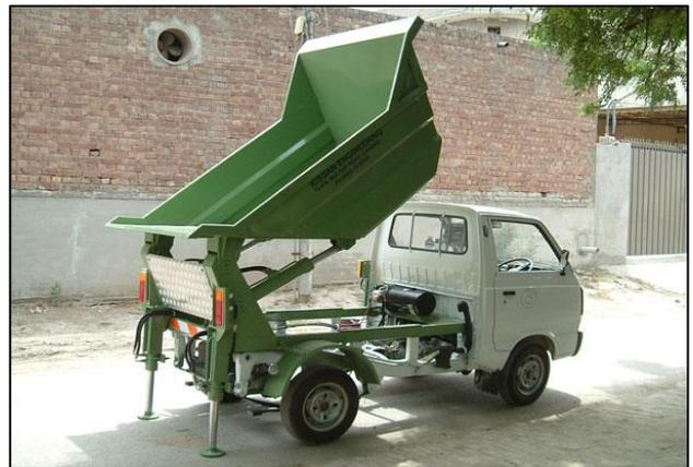
Container Hook Lifting type Mechanism
