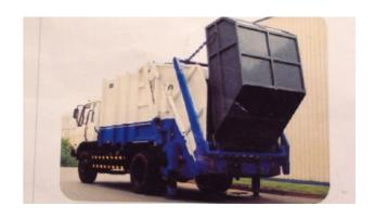
Bucket tipping mechanism-A4 Appliances- special metal covering bucket.
